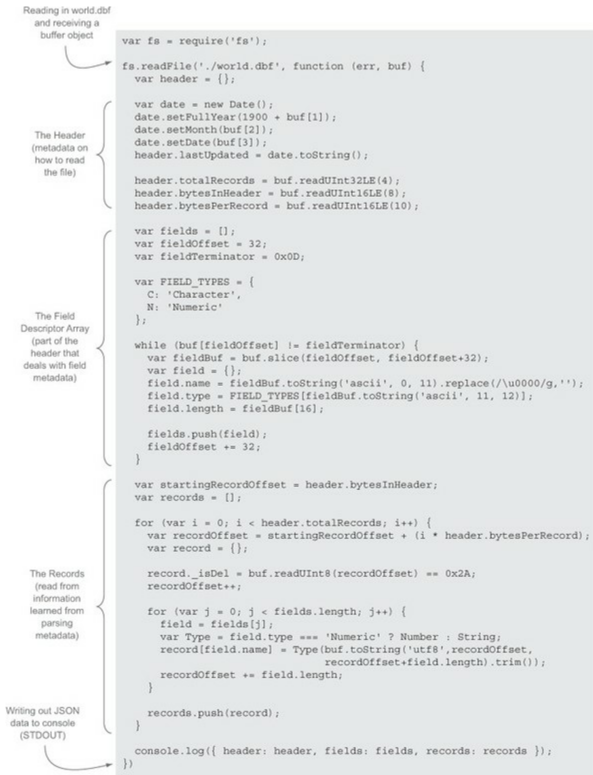
Figure 3.9. The full set of code for parsing a DBF file into JSON
